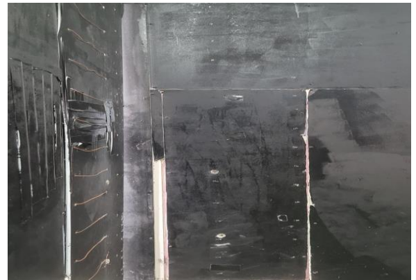
Fig 4 TC and HFG on Section Wall
